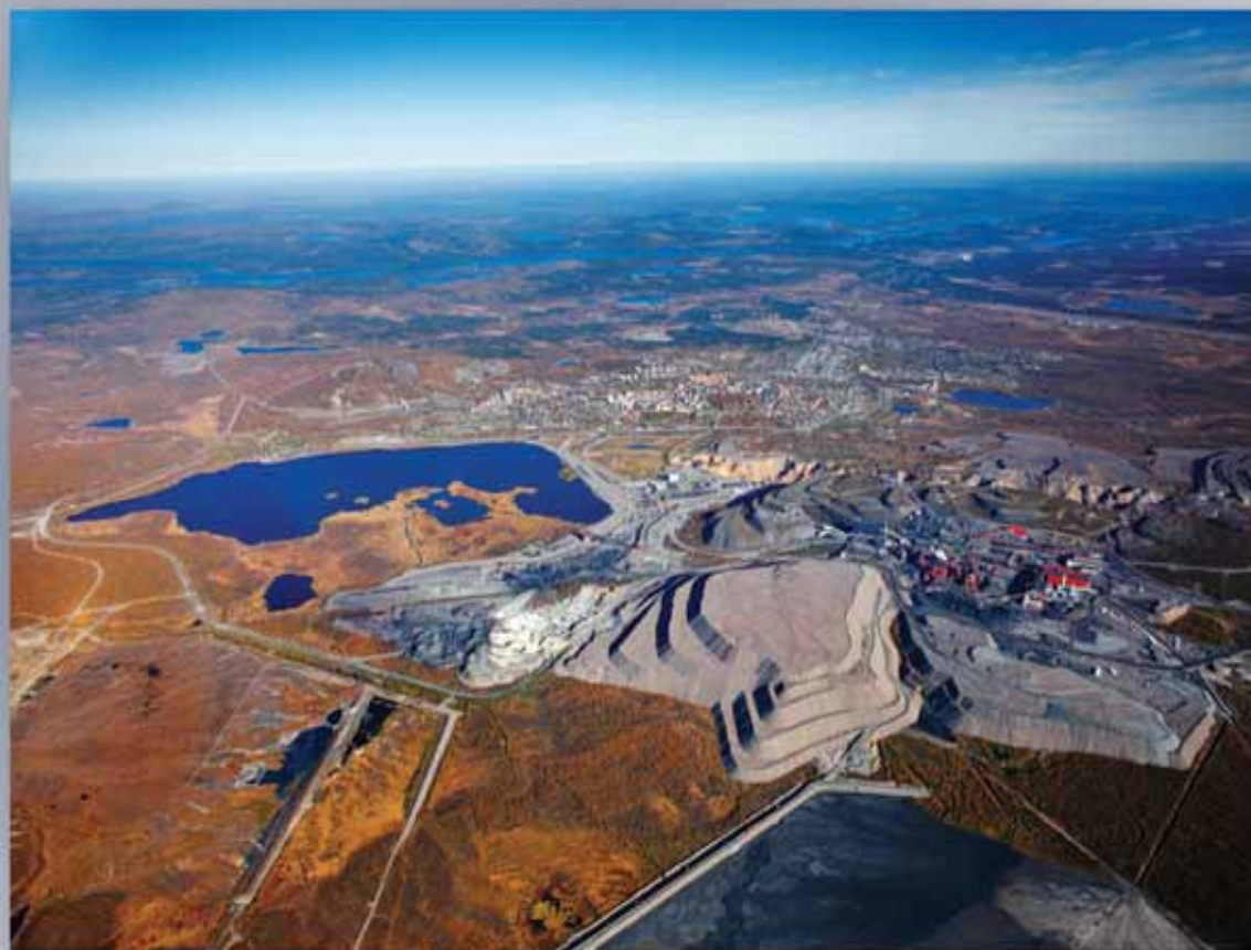
The industrial area at LKAB's Kiruna mine, with waste rock dumps and tailings.
